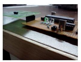
modulator/demodulator, we soldered the circuit on general purpose PCB.
