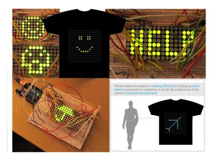
In the next version, we will use the below LED panel for display instead of LED matrix. One of the other goals of this work is to try to come up with a flexible display which can be stuck anywhere from clothes to bags to furniture.
