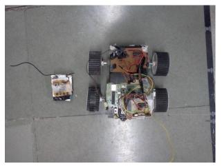
The task was to wirelessly control a robot and move it around. To achieve this task, I made use of 315 MHz RF transmitter and receiver modules. I used HT12E encoder chip and connected it to 4 push button switches. The data out was connected to the 315 MHz transmitter. The receiver was kept on the robot and was connected to the HT12D decoder chip. The output of the decoder chip was given to the microcontroller.
